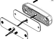
3. Remove the outer housing of the Versa Star<sup>®</sup> light and attach the light to the BB274-FISUV-VER bracket using the screws that came with the light.
