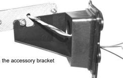
5. Poke a small hole in the rubber plug on the accessory bracket and route the wires through it.
